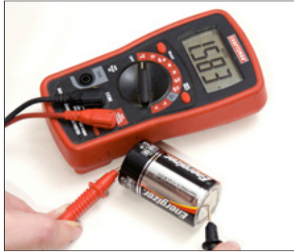
9. To measure the voltage of a battery or power supply, the probes are touched to the positive and negative ends of the power source.
