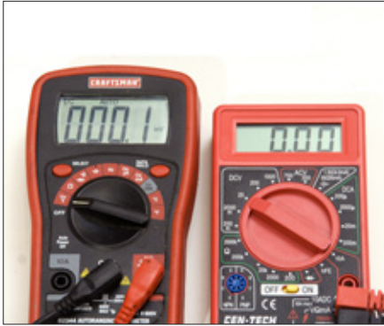
8. A side-by-side comparison of an autoranging (left) and traditional meter. Note that the autoranging meter will also automatically determine AC or DC voltage, as indicated by the icon with the straight line underneath the wavy line.
