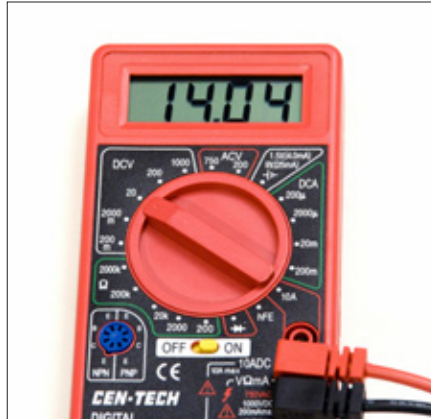
2. With a traditional meter, you must select from a range of values within which you believe your voltage, current, etc. might read. Here, the meter is set to 20V and displays the measured voltage (of a throttle) at 14.04V DC.
