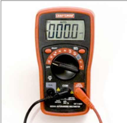
1. A multimeter has three basic parts: the display (digital shown), the dial (to select what you want to measure), and the probes (to connect to the component being measured.)
