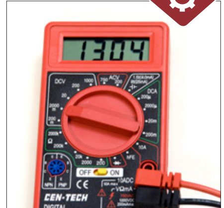
3. The accuracy of the value being displayed depends on the setting. In this example, the meter is set to 2,000 mV (2V). Reading a standard alkaline battery, it reads 1,304 mV, or 1.304V—accurate to a thousandth of a volt, as opposed to the hundredth shown in photo 2.
