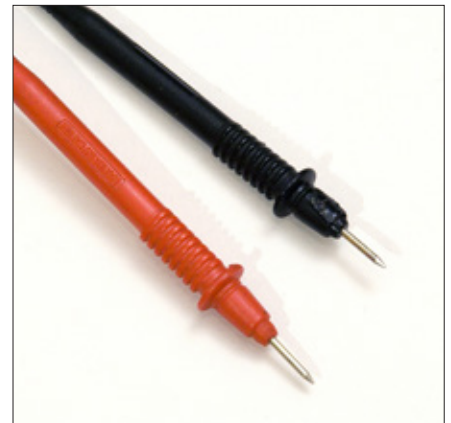
6. Probes connect the meter to the object being measured. Most meters come with simple probes, such as these. Other varieties can be purchased for specialized circumstances.
