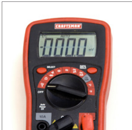
5. An "autoranging" meter will say "Auto" somewhere on the front of the meter or on the display. Also, you will not see any ranges from which to select; you'll simply see one setting each for voltage, current, etc.
