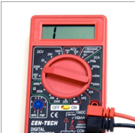
4. If the value measured is outside the meter's selected range, it will display an error message or similar, such as the "1" on this meter.
